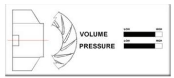
Backward Incline Laminar industrial fans are typically known as clean air fans and seen in spray booths as supply air fans. They are also used in ovens where pressure requirements are higher than normal. These impellers are efficient and therefore consume less power. Its inclined laminar blade can help any unwanted material to pass through its discharge even though it is not designed for conveying purposes.
