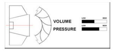
Even though this impeller is classified as a radial tip blade, it is urging on the forward curved style industrial fan. The modified blade allows this impeller and limited to conveying very light up to heavy dust and is ideal in the timber mill industry. The RBM fan runs at 2900rpm and is also quite noisy and inefficient, however a much preferred alternative to the RB.
