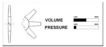
Tube Axial industrial fans are typically found in dry spray booths and are commonly uses for supply air and clean air exhaust applications. This impeller is easily designed for a wide duty range by simply setting the desired blade pitch and are manufactured in mild steel, stainless steel and can be sourced in a poly material as well. They are a relatively efficient option and therefore quiet.
