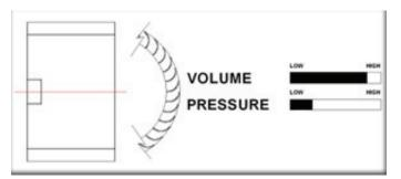
Forward Curved industrial fans are ideal for re-circulating large volumes of air with low pressure requirements. Slow revolving and not as highly stressed as an RB fan. Forward Curved industrial fans are normally used in the Furnace Industry for oven recirculation and drying. It is typical to find these fans belt driven and slowed down to under half speed of the motor driving it. These fans are not very efficient but are very quiet considering the amount of air they push.
