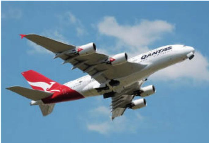
Considering the sheer size of the new Airbus A380, with a take-off weight up to 571,000kg, a wing span of 79.75m and a height of 24.45m, airports around the world needed to review all aspects of airport management to cater for this massive aircraft.
